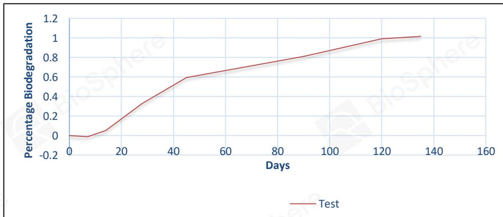
**Graph-2b: The percent biodegradation of the Test sample (Normal PET bottle + Lids Sample) determined based on conversion of carbon from the Test material to carbon in the gaseous phase (CH<sub>4</sub> and CO<sub>2</sub>)**
