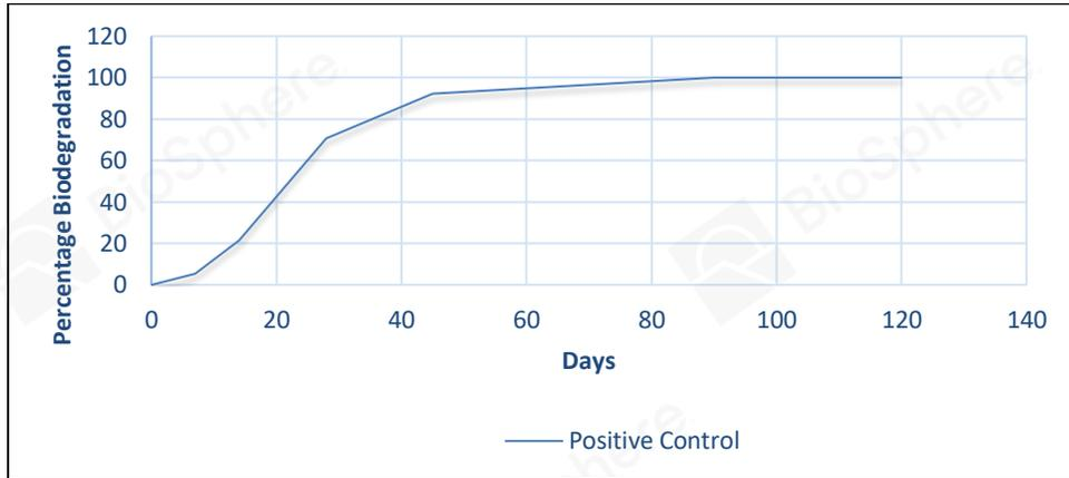
**Graph-2a: The percent biodegradation of the Positive control (Reference material- Cellulose) determined based on conversion of carbon from cellulose to carbon in the gaseous phase (CH<sub>4</sub> and CO<sub>2</sub>)**
