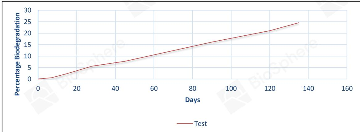
**Graph-2c: The percent biodegradation of the Test sample (PET + Biosphere (1%) (No Lid) Sample) determined based on conversion of carbon from the Test material to carbon in the gaseous phase (CH<sub>4</sub> and CO<sub>2</sub>)**
